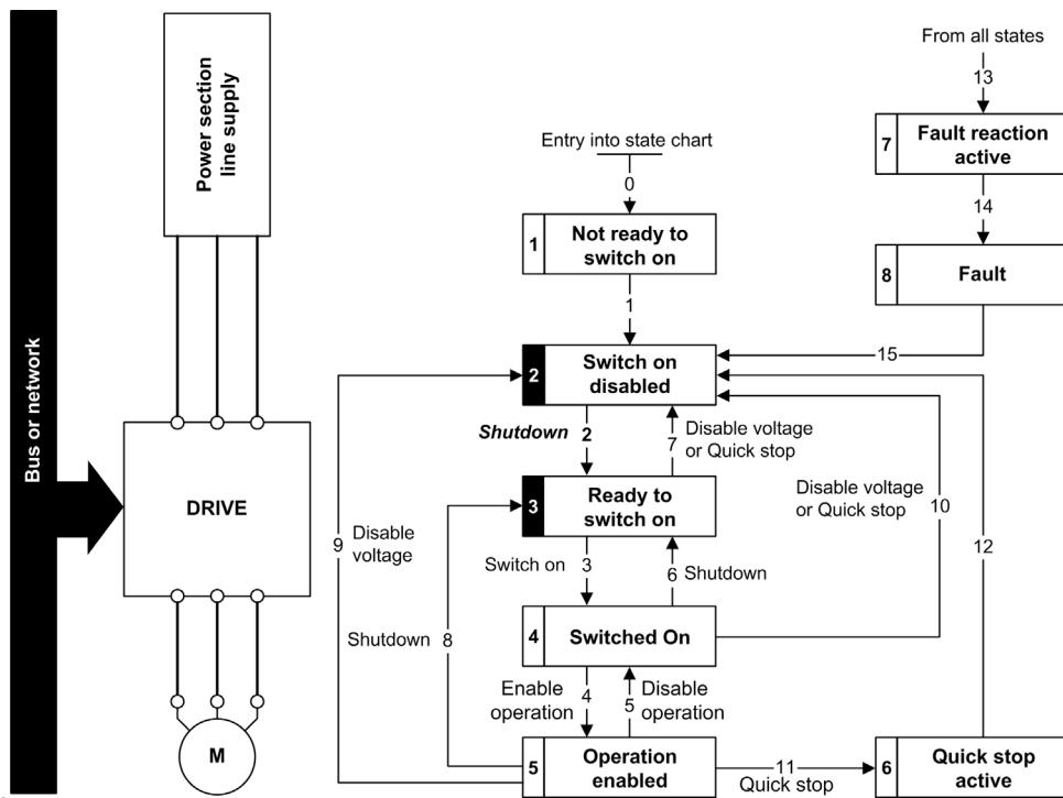
3. Verify that the drive is in the [3 - Ready to switch on] state.
